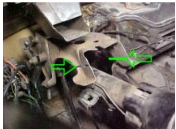
Cut the steering column tabs off the new pedal assembly
