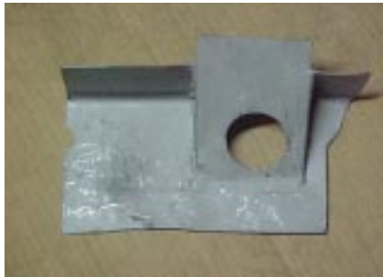
Clutch cable bracket ~ to hold the fire wall adjuster and cable.
