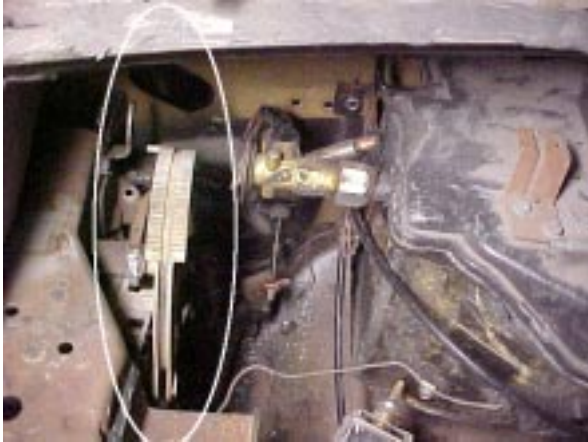
Quadrant next to evaporator box and expansion valve
