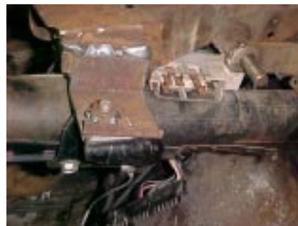
Shows where to cut to clear the ignition switch
