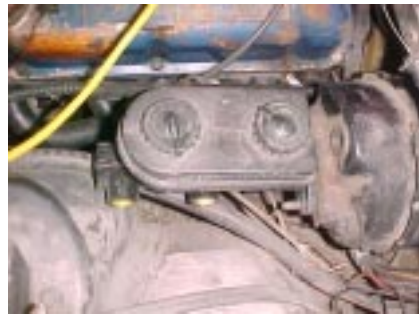
new big bore custom master cylinder and new (used) booster in place.
