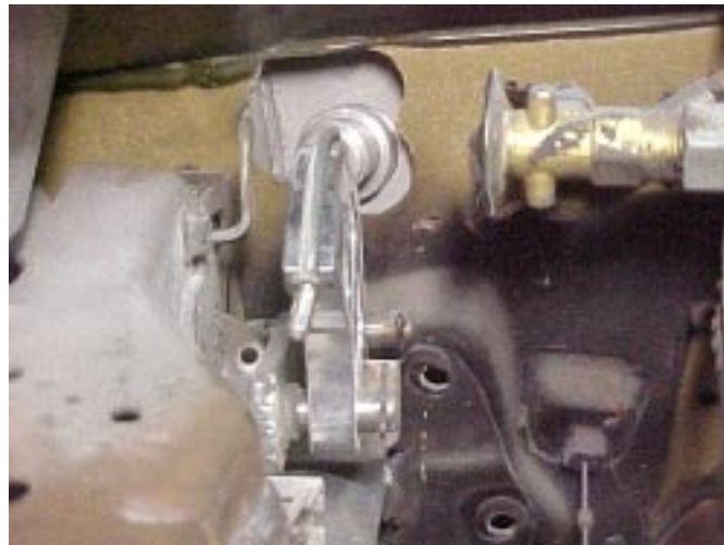
As seen from the inside of the car, note the extra trimming on the firewall, this was excessive but part of the cut and paste trial and error
